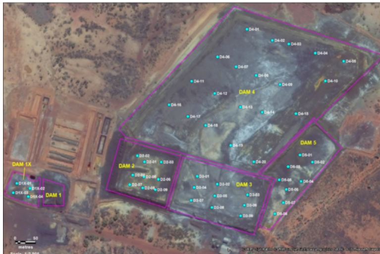
Figure 1: Map of the Peko tailings showing distribution of the drill holes drilled in 2016
