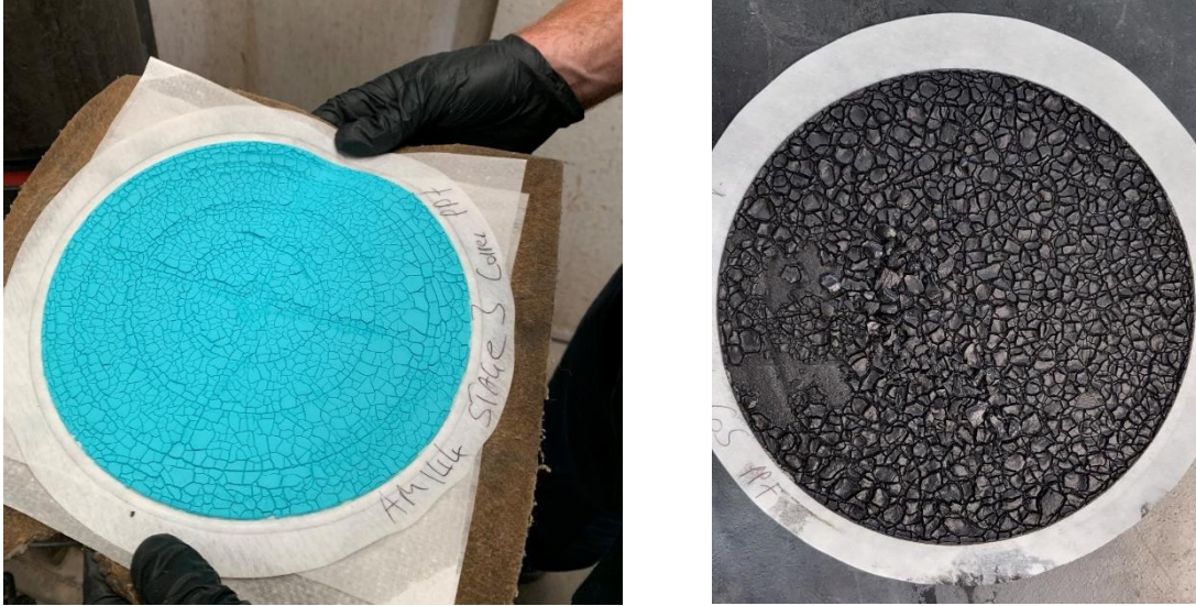
Copper carbonate (left) and cobalt sulphide (right) products made by Elmore in the laboratory using Peko soluble metals
