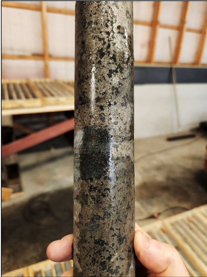
Figure 2: Coarse Ni-Cu-Co bearing magmatic sulphides from hole 21DDTS007 into the Granmuren Intrusion. The semi-massive sulphides towards the base of the intrusion contain rip-up clasts (large dark patch in centre of core) which are caught up in the sulphide mush during emplacement of the intrusion into the country rock sediments. This provides evidence that the drilling is getting close to the base “keel zone” of the intrusion where massive to semi-massive sulphides typically accumulate.
