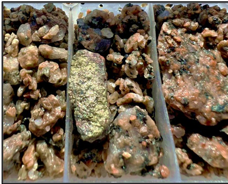
Figure 1. Chalcopyrite in potassic altered granodiorite from the Bank prospect (96-99m, 22BKRC003).
