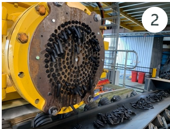
Photos: (1) Yallourn brown coal (lignite) being loaded to the infeed system, (2) achieving COLDry pellets on the first end-to-end wet commissioning run of the primary processing system & (3) dried pellet samples.
