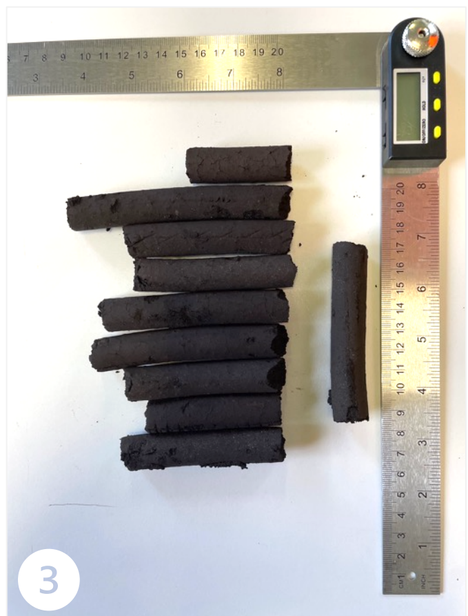
Photos: (1) Yallourn brown coal (lignite) being loaded to the infeed system, (2) achieving COLDry pellets on the first end-to-end wet commissioning run of the primary processing system & (3) dried pellet samples.
