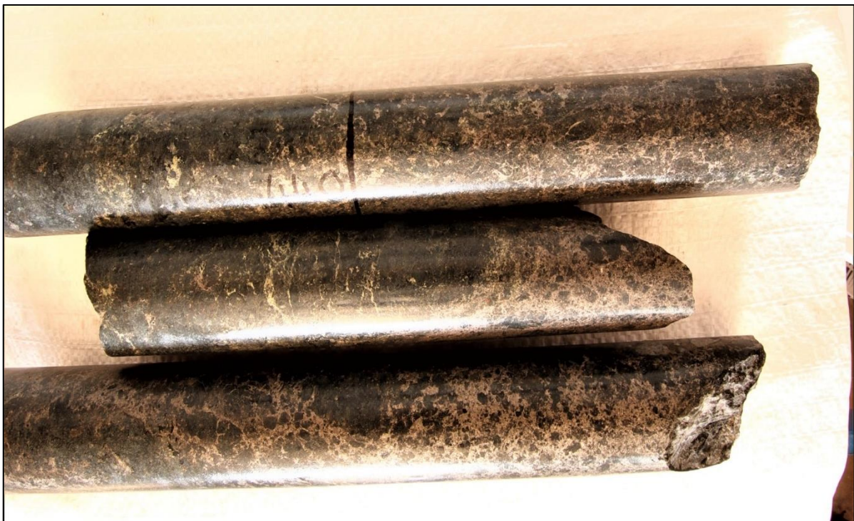
Image 1: Semi-massive and matrix nickel and copper sulphide mineralisation at 440m in hole ANDD0172 (within a strongly mineralised 24.6m interval)
