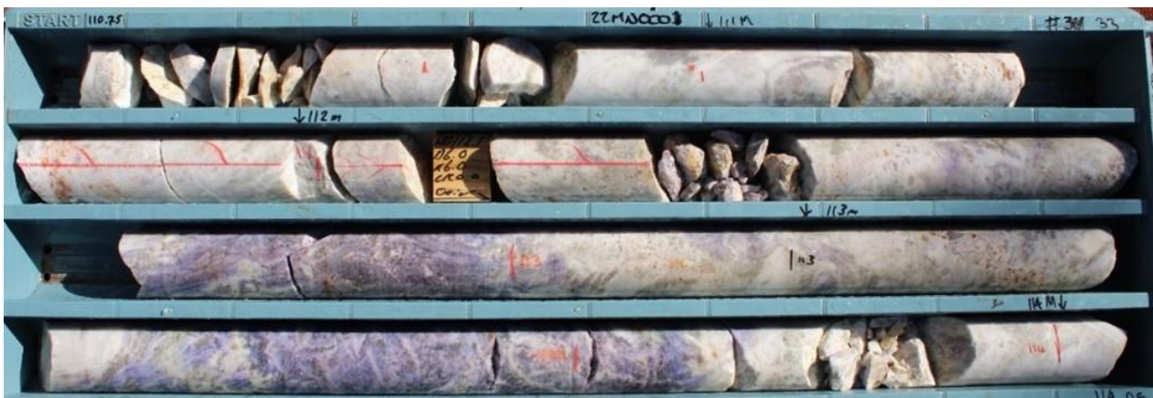
Photo 1: Foundation Pegmatite 22MNDD001 lithium bearing drillcore 111 – 114m (lepidolite +/- spodumene)
