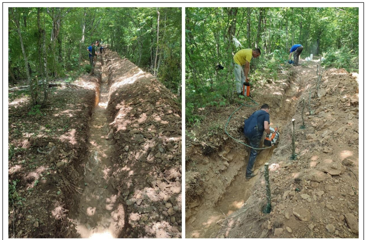
Figure 6: Zekil-Erak Prospect – trench SICH001 and sampling with handheld rock saw
