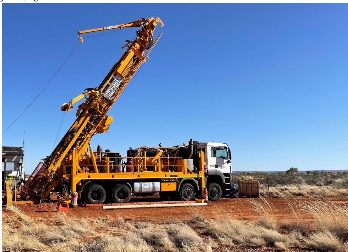
Figure 1. Diamond Drilling underway at the West Tanami project.
