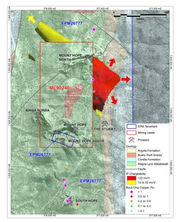
**Figure 1.** Mount Hope EPM26777 showing the vertical plan view of the processed chargeability response at the +14mv/V and +22mv/V levels.
