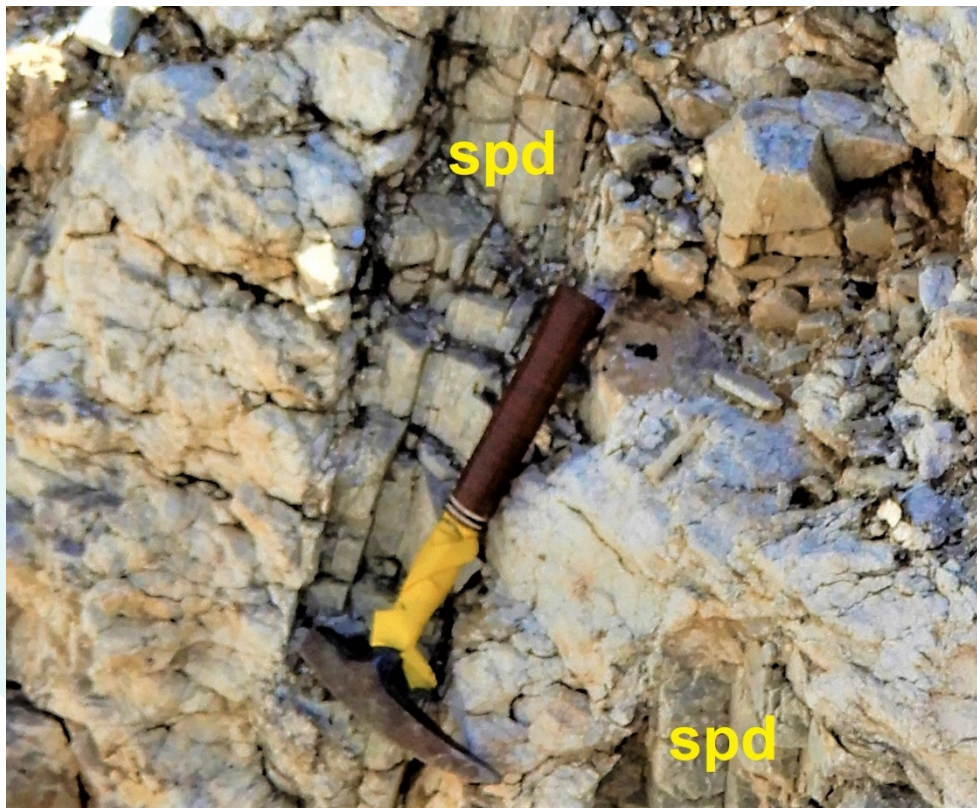
Figure 5: Spodumene crystals, labelled spd, exposed at 226120mE/8323015mN (WGS-84 z33L) in wall of a small trench in a pegmatite within the Namibe Lithium Project.
