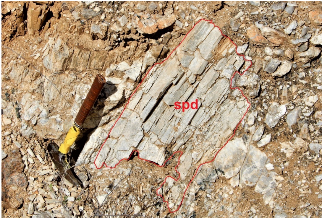
Figure 6: Spodumene crystal (outlined in red and labelled spd) at 226115mE/8323024mN (WGS-84 z33L), site 19a. Sample AAR013 was taken from this location.
