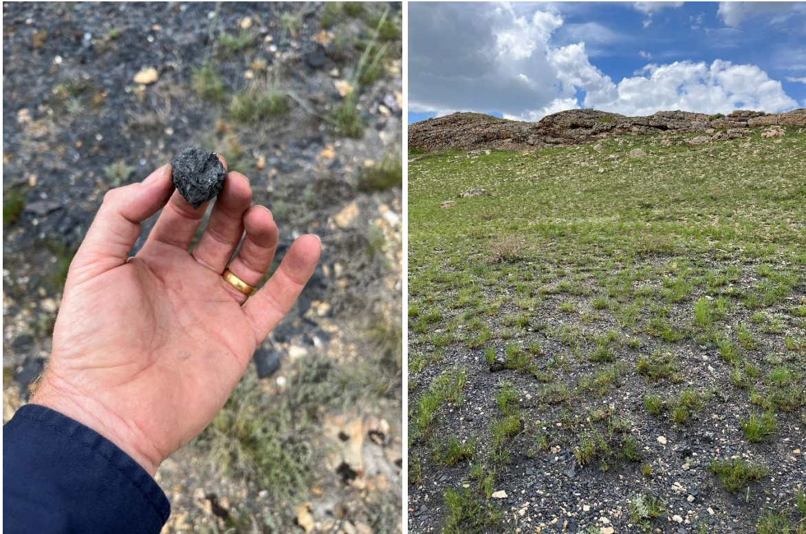
Figure 4 - Coarse graphite crystals at the outcrop between the granite dome intrusion and graphite mineralisation to the east of the Central Graphite Zone, outside of the current Mineral Resource. Photos looking north-west at approximately 440000mE 5375000mN.
