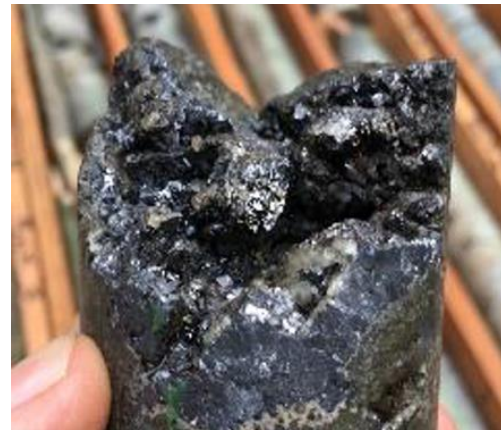
Coarse galena and sphalerite within a breccia unit
