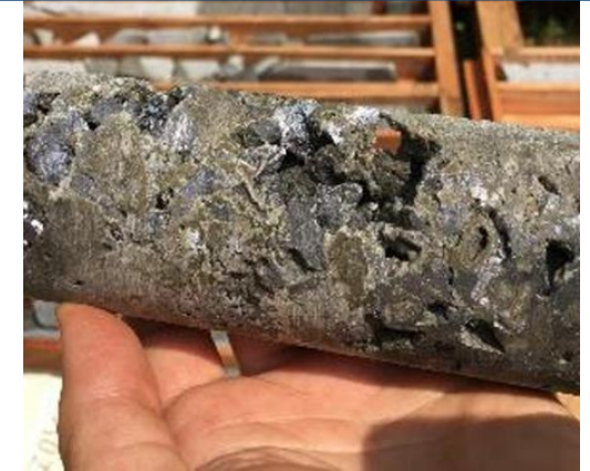
Coarse textured galena, sphalerite and marcasite within the basal carbonates unit
