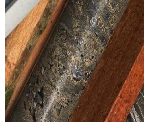
Concentric textured sphalerite and coarse galena within a breccia unit
