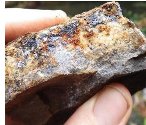
Carbonate hosted displaying coarse galena crystals
