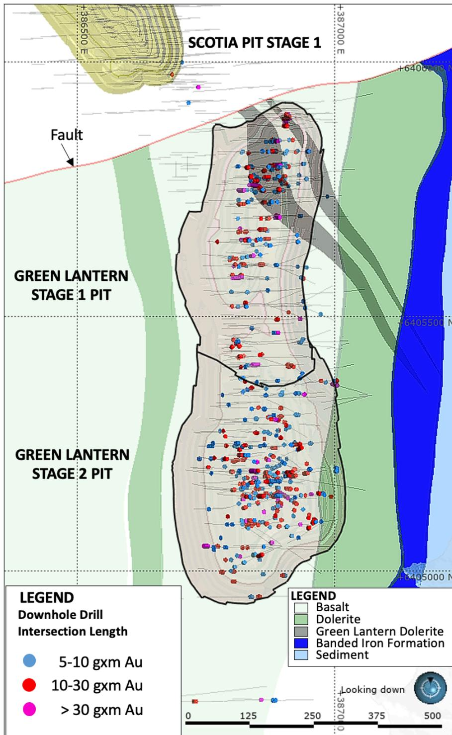
Figure: Plan of Drilling and Pit Designs at Green Lantern.
