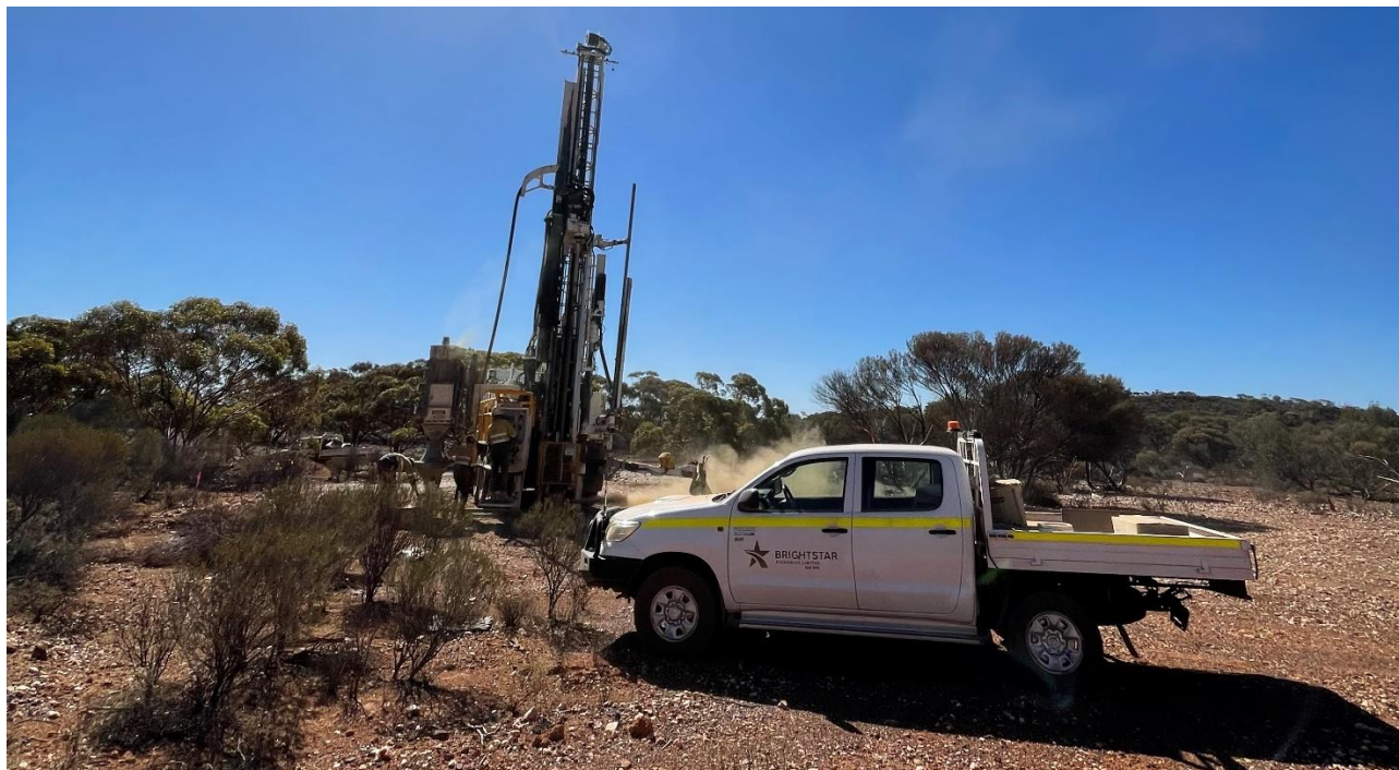
Figure 1: Aircore Drilling at Sailor Prince prospect.
