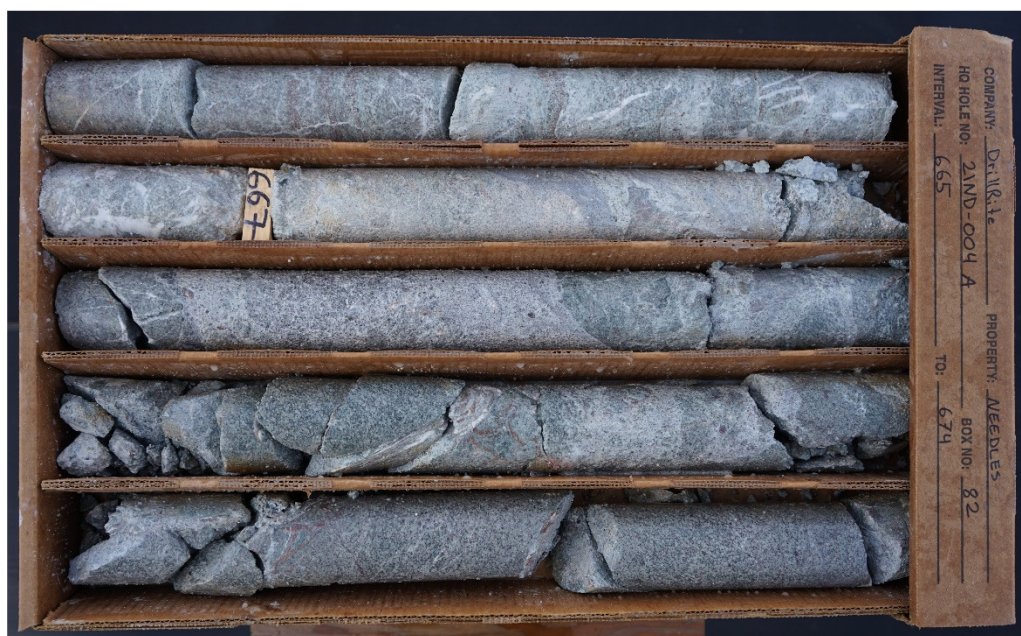
Figure 4. Example of latite-andesite tuffs in hole 21ND_004A Box 82 from 665 to 674 feet (202.7 to 205.5m) - phyllic altered andesite and latites with disseminated pyrite [+2%].
