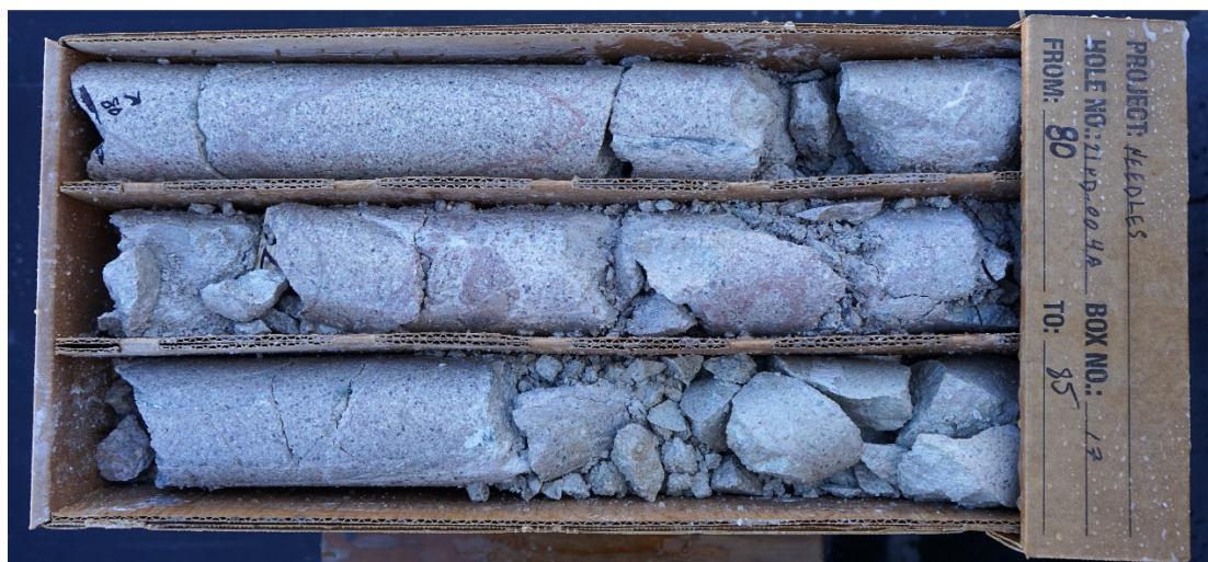
Figure 3. Example of pyrite/hematite veined dacitic crystal tuff in hole 21ND_004A Box 17 from 80 to 85 feet (24.4 to 25.9m) - propylitic altered andesite and dacites with disseminated pyrite [1-2%].
