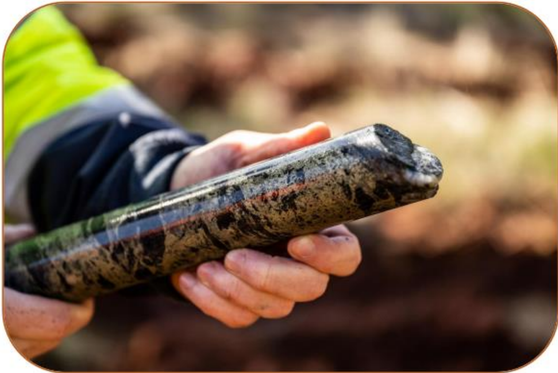
Figure 5: CANDD011, interval of semi-massive chalcopyrite with approximately 20% of chalcopyrite from 152m
