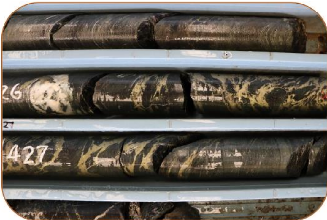
Figure 6: CANDD012, interval of chalcopyrite veins in chlorite altered pelite from 426m
