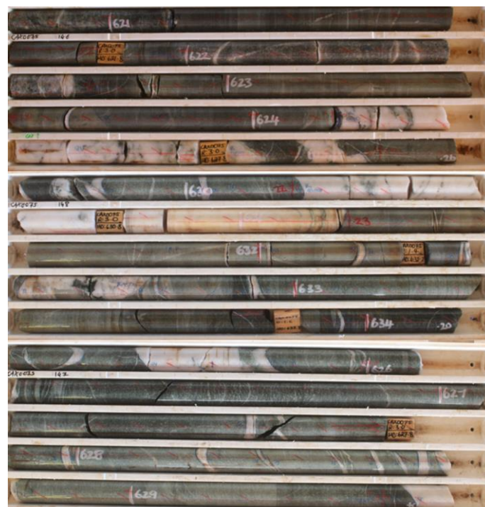
Figure 8: EIS Hole CAX0075 showing mineralised intersection on the Lords Fault (one of the main controlling faults for Darlot mineralisation).
