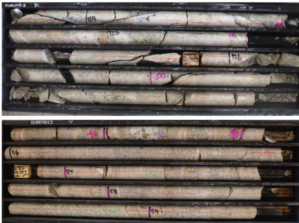
Figure 6: KHRD0602 & KHRD0623 – strongly mineralised tension veins in the Central area within the granodiorite (down hole drill metres in black).
