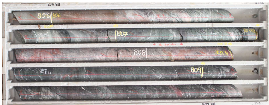
Figure 2 - Drill core showing alteration and lithology logged around the trace/minor bornite mineralisation within exhalative sediments at 808m. Size of drill core = NQ or ~47.6mm.
