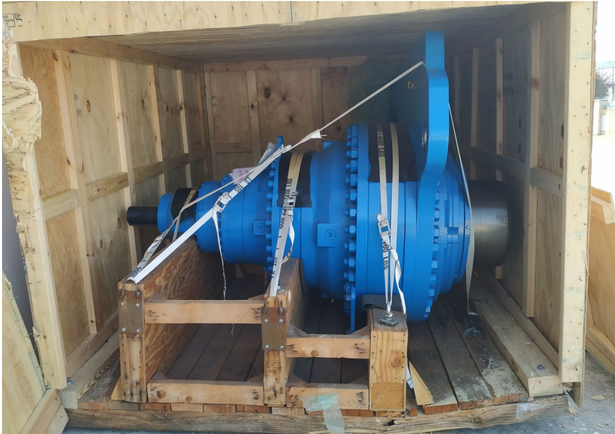
FIGURE 11: LUDMAN INDUSTRIES COMPACTOR GEARBOX FOR PROCESSING PLANT ON-SITE IN SPAIN
