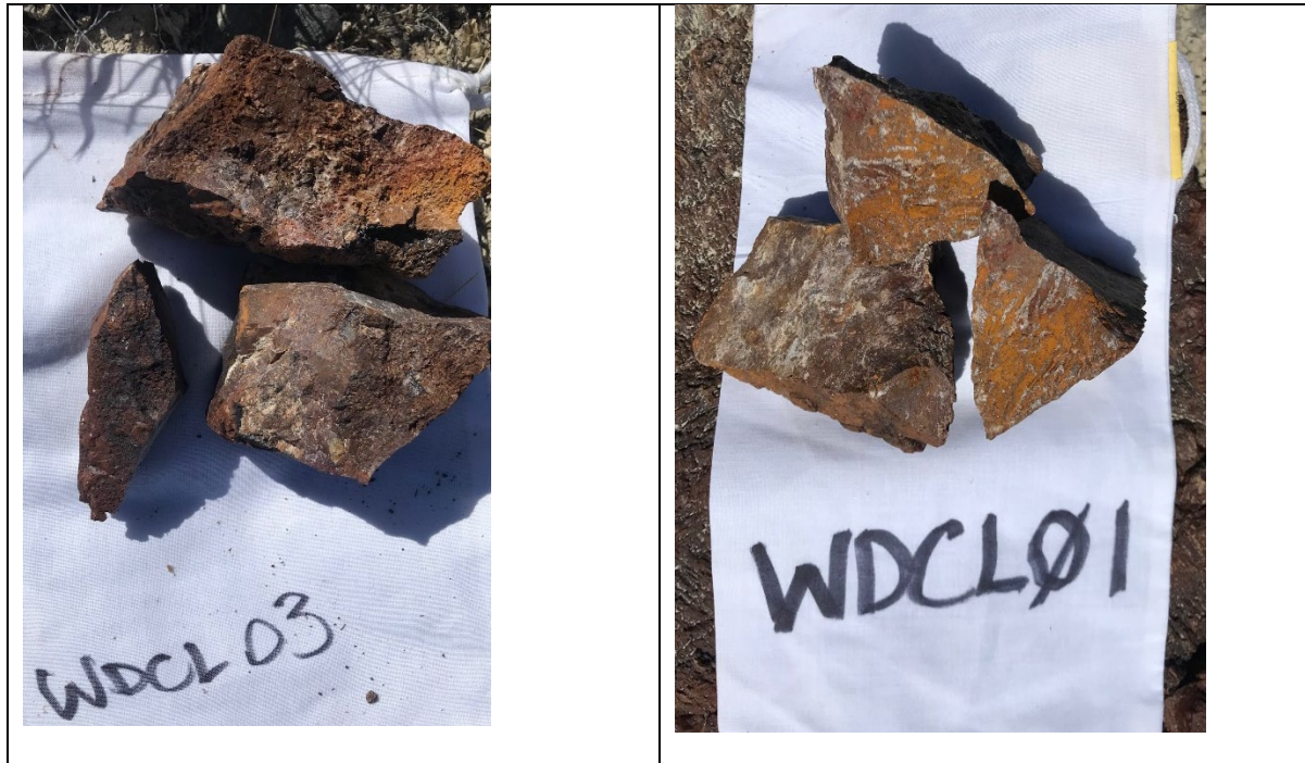
Figure 9- Rock Samples WDCL03 (0.95 g/t Au) and WDCL01 (0.26 g/t Au)- Red- red brown highly siliceous altered limestones, A3N Prospect area.
