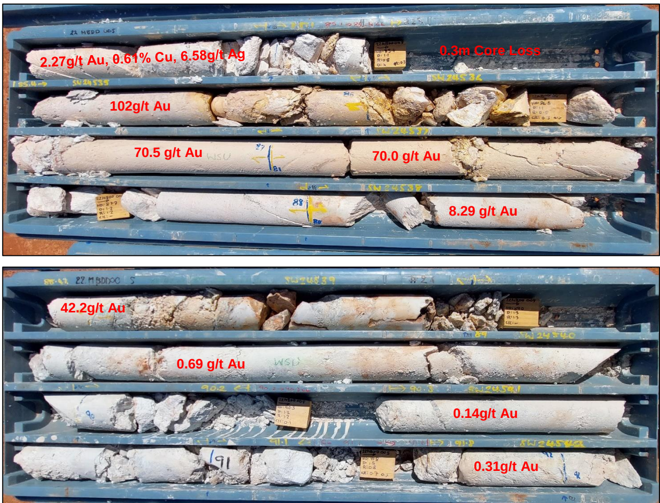
FIGURE 3: CORE PHOTOS THROUGH THE MINERALISED ZONE IN 22MBDD005.
