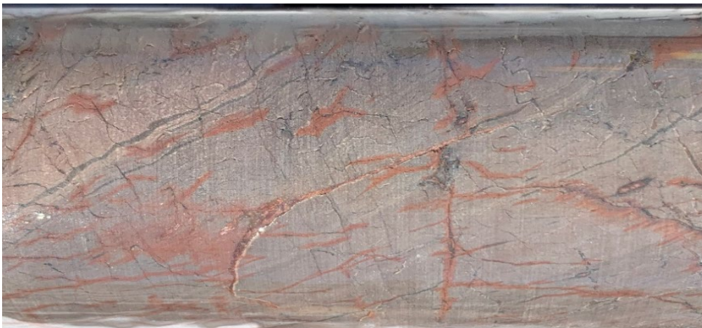
Figure 5: Hematite alteration 'bleeding' out from microfractures in metasediments. Hole Depth 298.7m.
