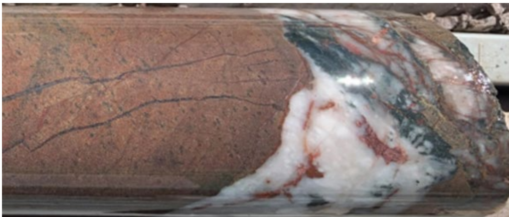
Figure 6: Quartz-chorite hematite vein metamorphosed lithic sandstone. Hole depth: 338.4m.
