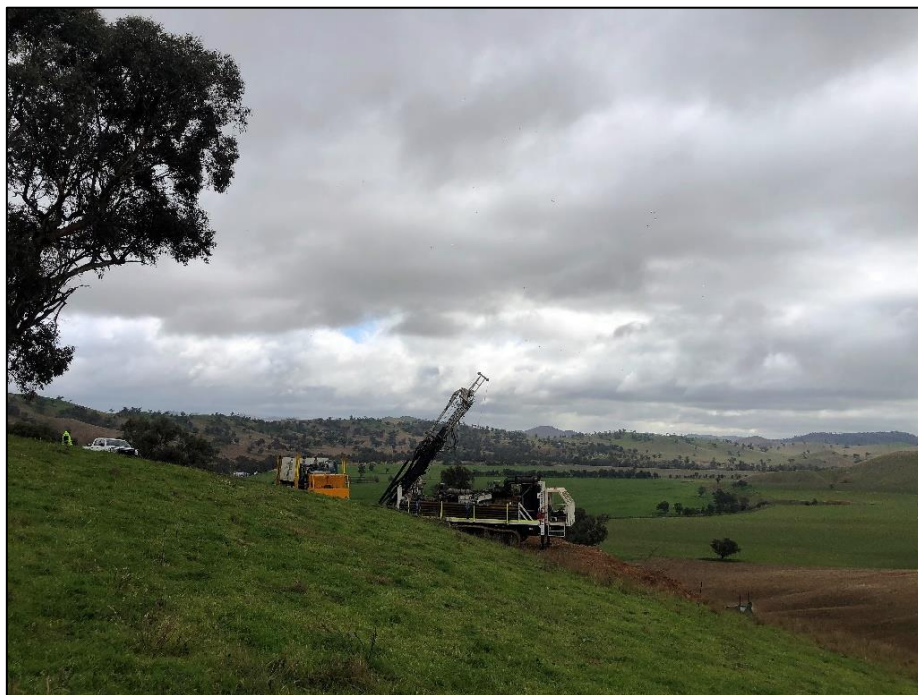
Figure 4: Photograph of the UDR650 track mounted drill rig on the first drill pad.
