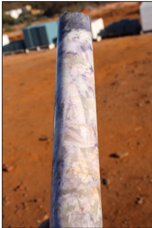
Figure 3: Drillcore photos from SPEX020 displaying extremely coarse spodumene (424.8m Photo1 and 436m Photo2 downhole) #
