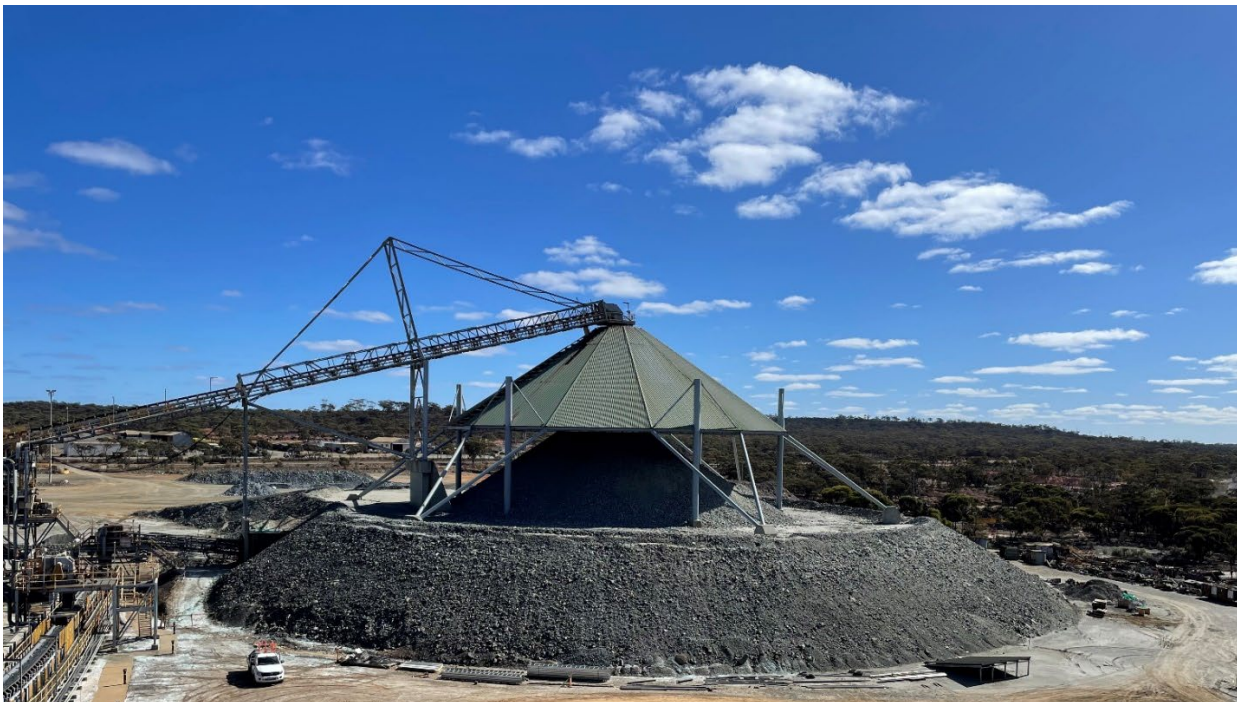
Figure 6: Mincor Ore in Crushed Ore Bin at BHP Nickel West's Kambalda Nickel Concentrator
