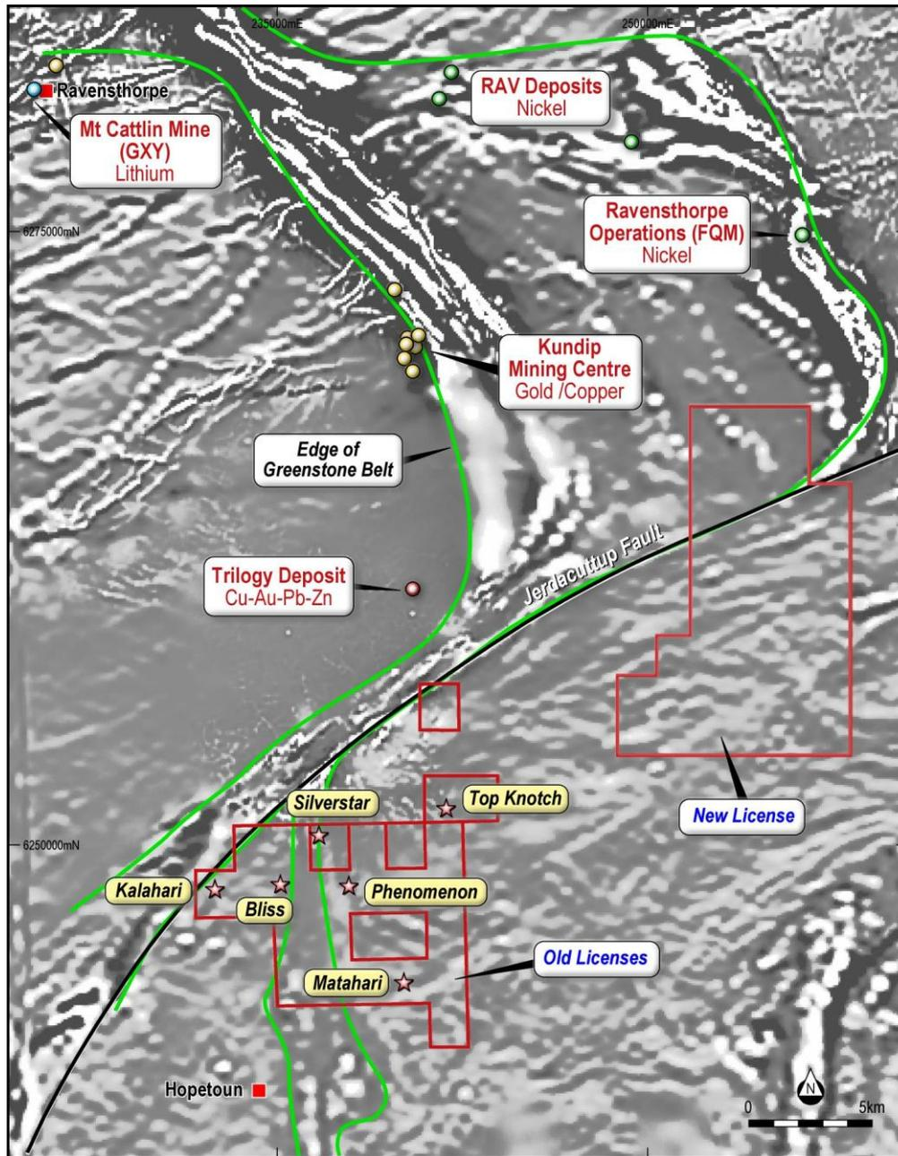
**Figure 3.** Image of airborne magnetic data over the Ravensthorpe-Hopetoun area showing the interpreted extension of the Ravensthorpe greenstone belt south of the Jerdacuttup Fault together with the licences in the Hopetoun Joint Venture. The new licence is EL74/730.
