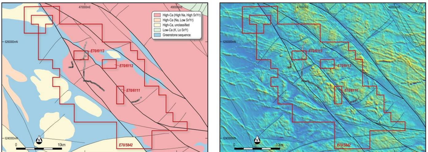
**Figure 5.** Geology of (left) and magnetic data (right) of the Dinninup Project showing major structures and the location of the soil geochemistry traverses.
