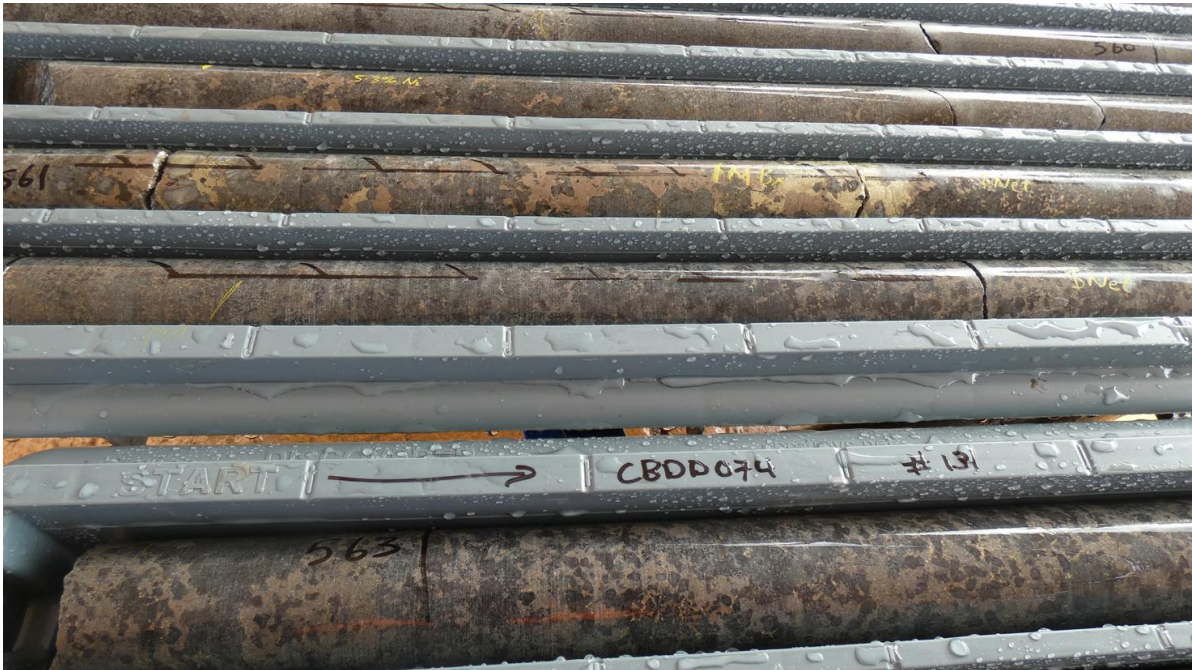
Figure 3: Breccia and matrix semi-massive nickel & copper sulphides from CBDD074 around 361m downhole depth
