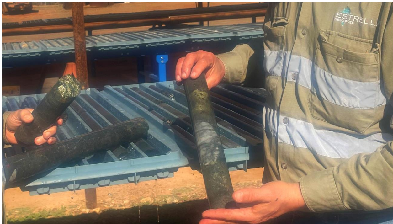
Figure 1: Mineralised core from CBDD076 at 415 - 420m downhole, showing nickel and copper mineralisation at Broonhill
