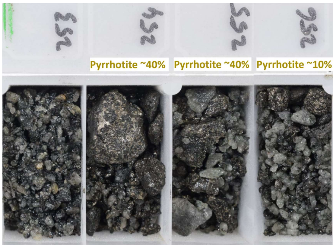
Figure 4: Drilling to a downhole EM target has intercepted a zone of semi-massive pyrrhotite 1 (BSRC1530 assays pending)
