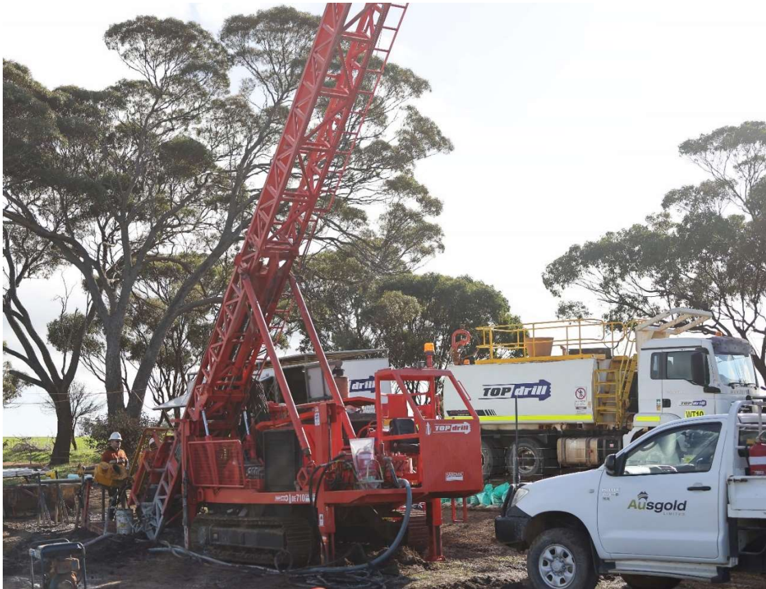
Figure 5: Diamond drilling targeting the EM plate in the down-plunge position north of the Jinkas high-grade zone (see figures 1 and 2)
