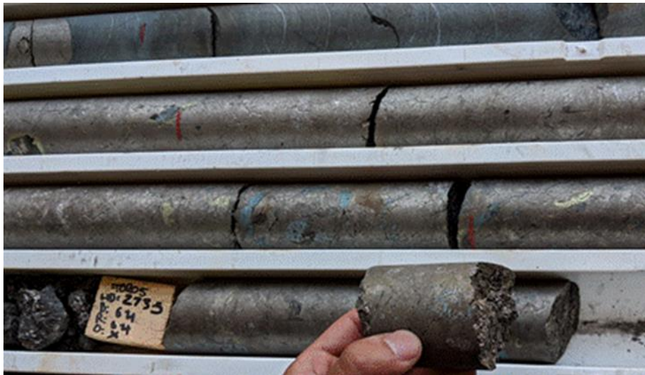
Figure Eight | Massive Sulfides in TOR05 from drilling at the Thor “Julimar lookalike” Target
