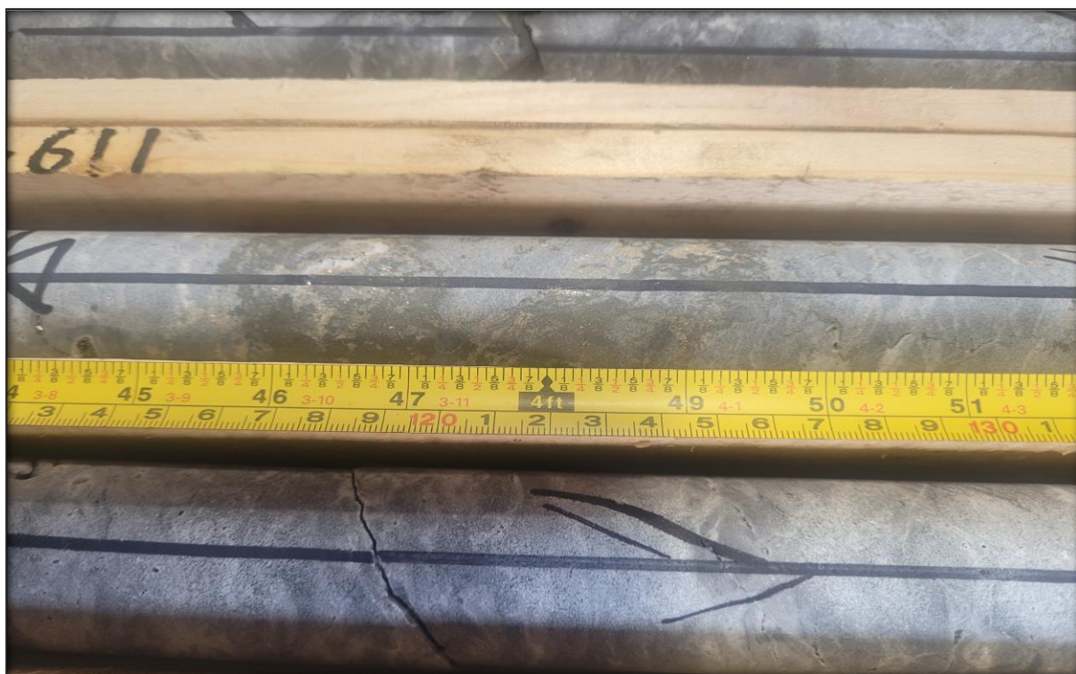
Figure 9. Drill hole RDD001 encountered a zone of fracture fill and stringer-style sphalerite, galena and pyrite between 597-612m and is currently awaiting assays.
