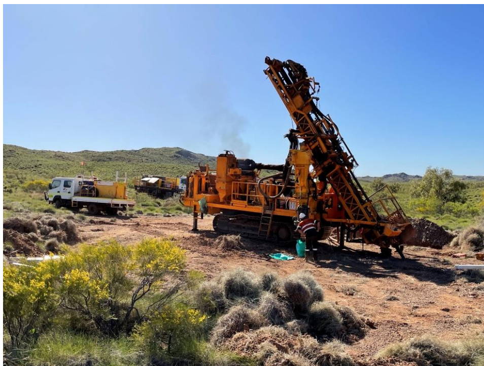
Figure 7: RC Drilling at Osborne Nickel Prospect
