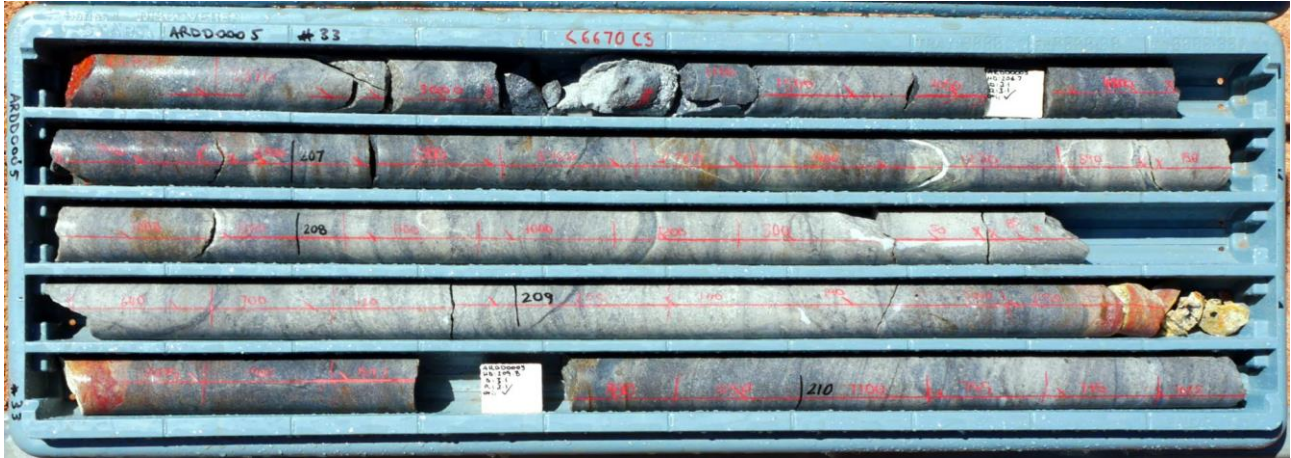
Figure 3: Typical high-grade mineralised veins in ARDD0005 drill core (206m – 210.4m), showing a combination of disseminated and fracture-controlled uranium mineralisation in a bleached silica-pyrite sandstone
