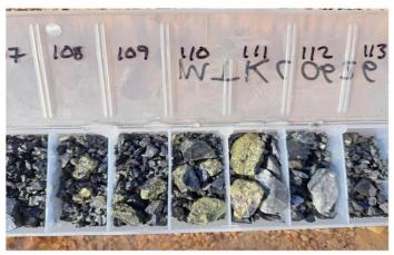
Figure 5. Lady Colleen MTKC00626 visible copper sulphides (tray108-111).
