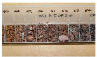
Figure 4. Lady Colleen MTKC00624 visible copper oxides.
