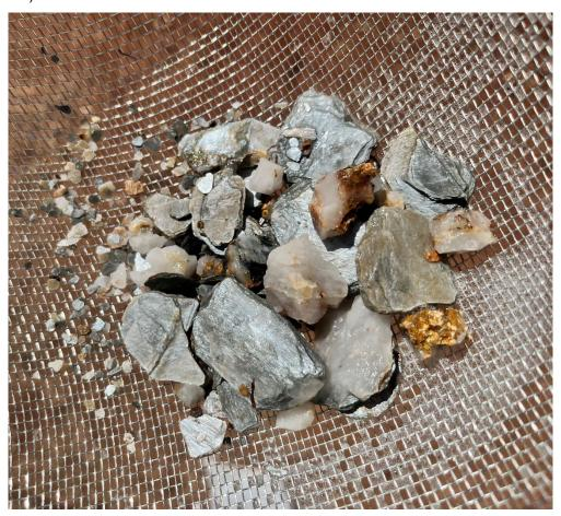
Plate 1 – Bottom of hole Chips in AHRC1076 – strong veining, shearing, alteration, and sulphide mineralisation – open at depth; 3m @ 1.59g/t Au from 68m.
