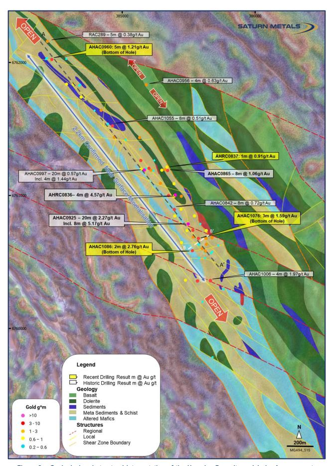
Figure 2 – Geological and structural interpretation of the Hercules Deposit overlain by Au gram metre values.  $^{(a) \, \text{Refer page 6}}$
