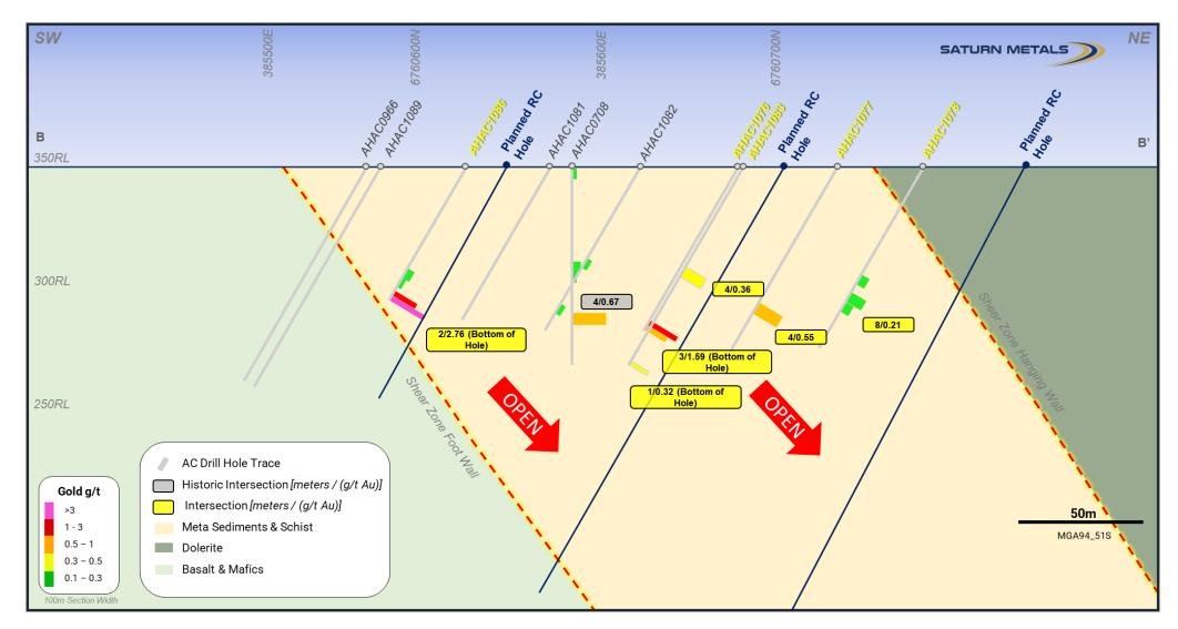
Figure 3 –Southwest – northeast cross-section B – B¹ location illustrated in plan view Figure 2 – Mineralisation contained within camp scale shear zone – drilling planned to target beneath the shallow anomaly which is open at depth. (a) Refer page 6
