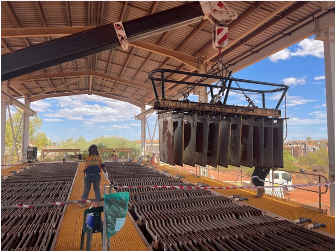
Image 4 / EW - Removal of Cathodes
