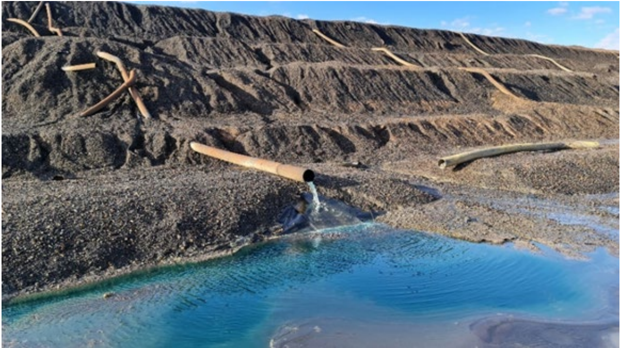
Image 14 / Copper rich solution flowing out of the heaps following recent rainfall at Nifty
