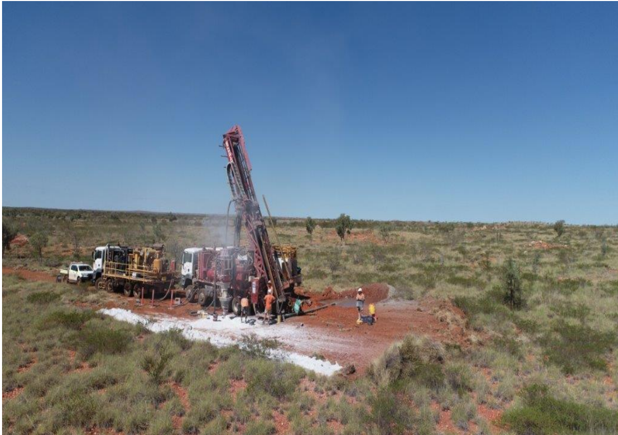
Photo 1 – FORACO Reverse Circulation Drill Rig at Shaw River historic Tin Tantalum Mine
