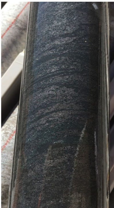
Figure 1. Semi-Massive to Matrix Magnetite Ore
