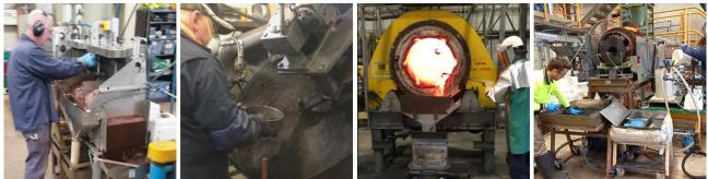
Figure 4 - AVL's process includes reverse flotation, pelletisation, salt-roasting and leaching; demonstrated at full pilot-scale from left-right
