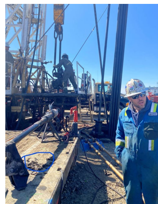
Workover completed at 2-29 to increase water disposal capacity to >12,000 bbl/d
