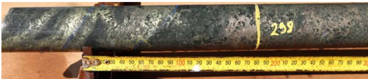
Figure 2. HMLVDD001 at 258m down-hole. Example of chalcopyrite-pyrrhotite mineralisation encountered in the hangingwall sulphide zone at Ajax east. Refer ASX announcement 29 June 2022.
