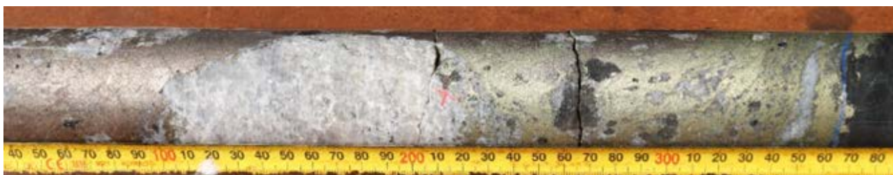
Figure 3. HMLVDD001 at 342.7m down-hole. Example of chalcopyrite-pyrrhotite mineralisation encountered in the footwall sulphide zone at Ajax east. Refer ASX announcement 29 June 2022
