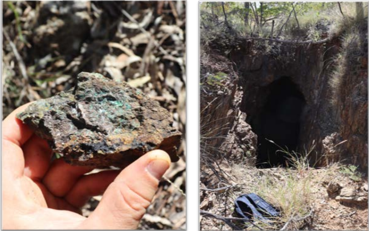
Figure 15. Copper workings and copper oxide mineralisation at Pearl
