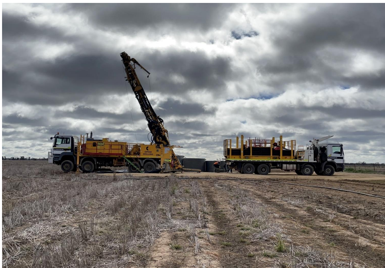
Figure 5. Diamond drill rig set up to drill hole the first hole of the 2022 program at the Myall Project, targeting porphyry-associated copper, gold and molybdenum mineralisation at the Corvette Prospect (ASX MAG 28 July 2022).
