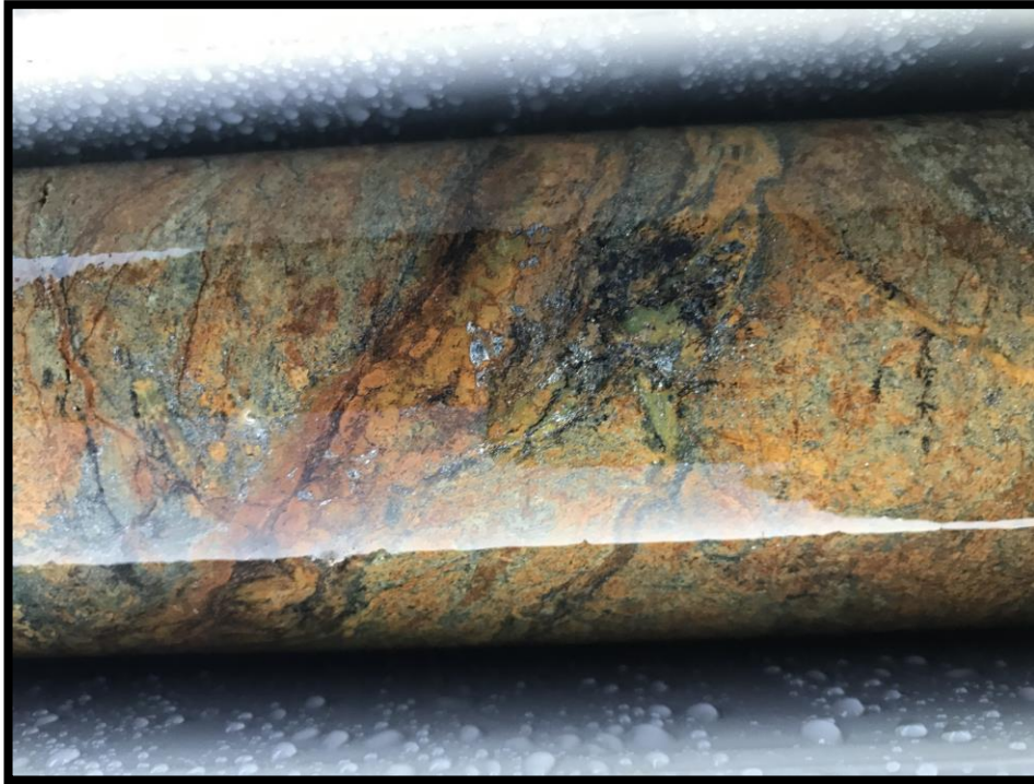
Figure 7 - Oxidised ultramafic in drill core (below surface gossan) (NRDD005) testing down-dip of the Dease Gossan (27.8m)
