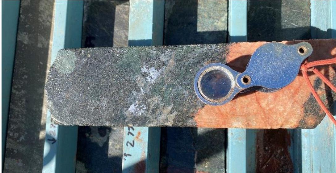
Photo 4: 21MHDD02- 282-283m (282.4m) - 1m @ 0.02% WO 3 , 0.23% Mo & 0.07% Cu - coarse grained visible molybdenite in magnetite skarn
