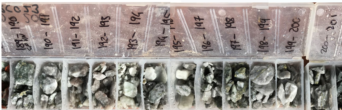
Image 1. MHRC023 Chip Tray showing 12m downhole copper sulphide quartz vein.
