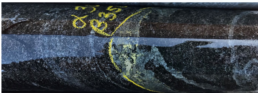
Image 2. LFDD142 core from 277.45m to 277.6m showing stringer veining mineralisation.
