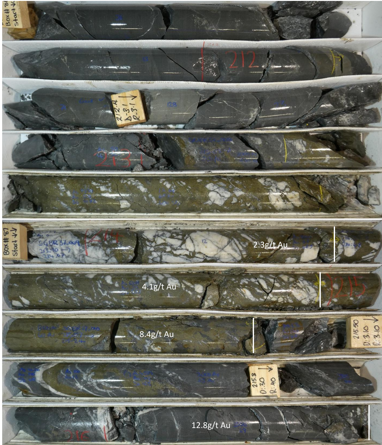
Figure 10. A2 shoot intersected in BR37. Quartz and pyrite breccia in the hangingwall with higher Au grades in the footwall acicular arsenopyrite mineralisation.
