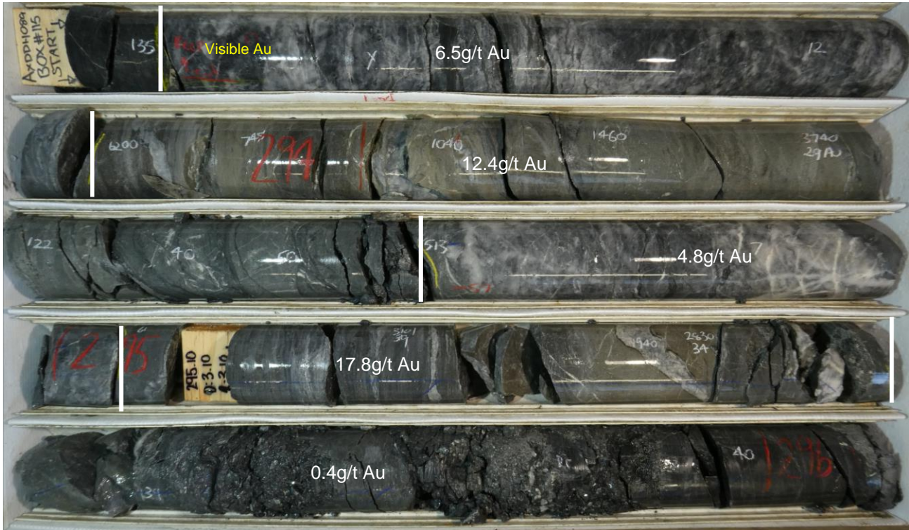
Figure 5. AX89 intersection in the McVicar West shoot: 2.3m @ 10.2g/t Au.
