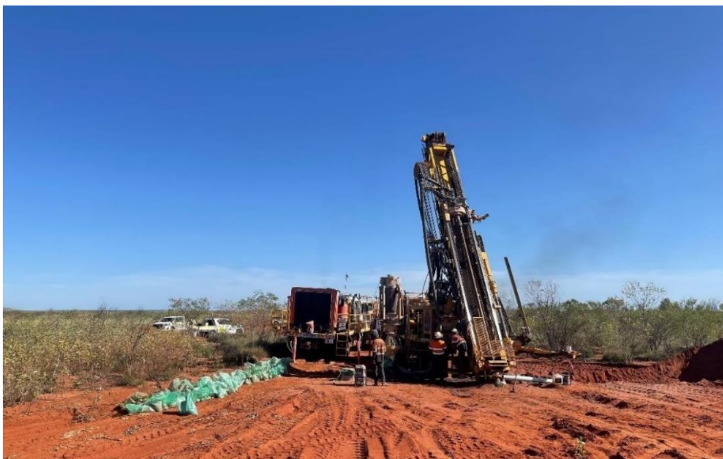
Figure 4: RC drilling at the Highway Ni-Co-Cu-Pd deposit.
