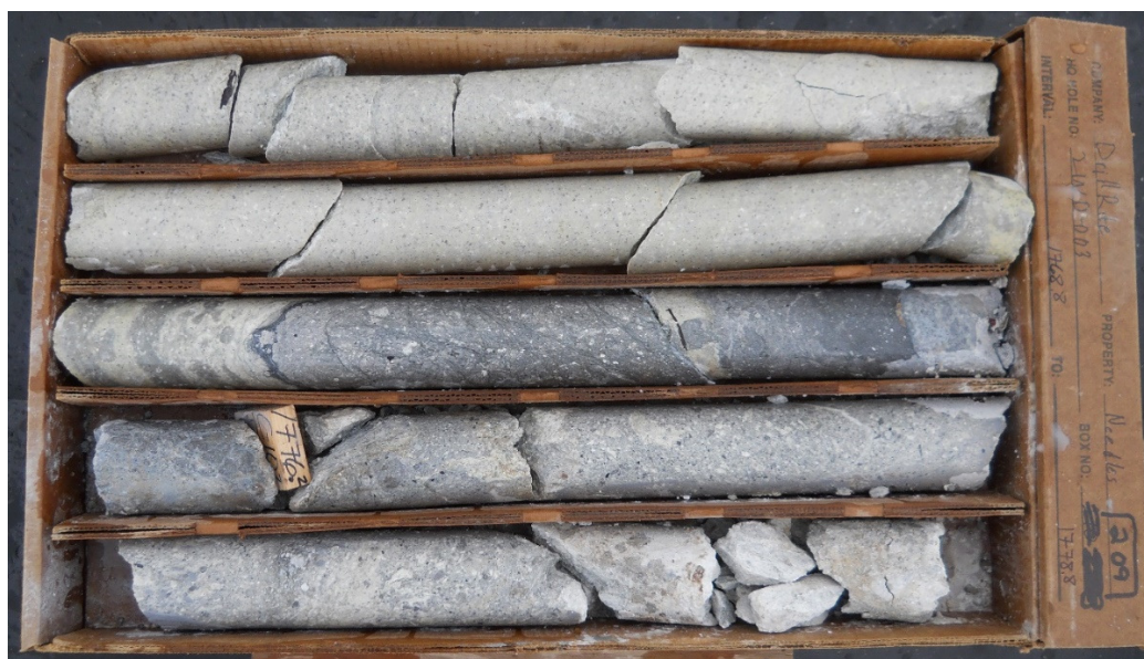
Figure 12. Example of pyrite veined andesite in hole 21ND_003 Box 209 from 1,768.8 to 1,778.8 feet (539 to 542m) – propylitic altered andesite and dacites with disseminated pyrite [1-2%].
