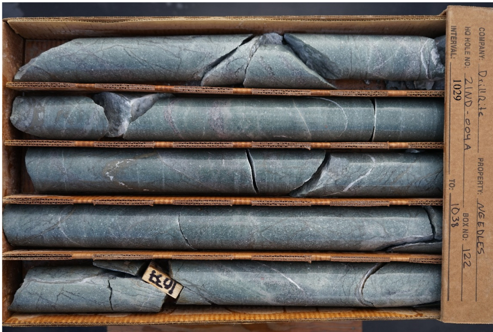
Figure 13. Example of pyrite veined andesite in hole 21ND_004A Box 122 from 1,029 to 1,038 feet (314 to 316m) - showing green propylitic altered andesite with brassy metallic veins of pyrite
