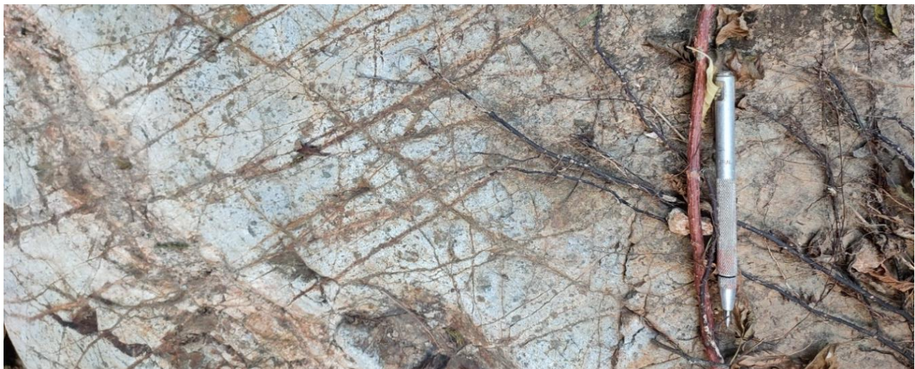
Plate 3. Kaliman Porphyry Target: Outcropping hornblende diorite with a stockwork of B-type quartz veinlets (millimetric quartz veinlets with iron oxides and sericite alteration halo) and thin magnetite veinlets.
