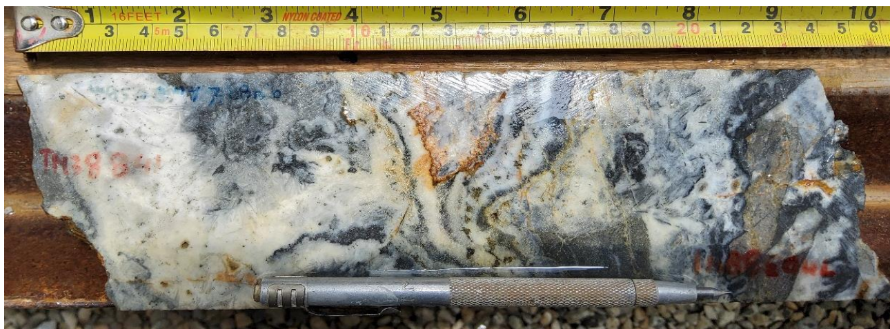
Plate 1. Foto Target: Quartz vein with colloform and replacement textures, mineralisation includes pyrite, arsenopyrite, and sphalerite.
