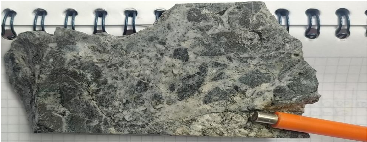
Plate 2. Comanche Target: Quartz vein with brecciated texture, mineralisation includes pyrite, arsenopyrite and chalcocite with associated supergene malachite.
