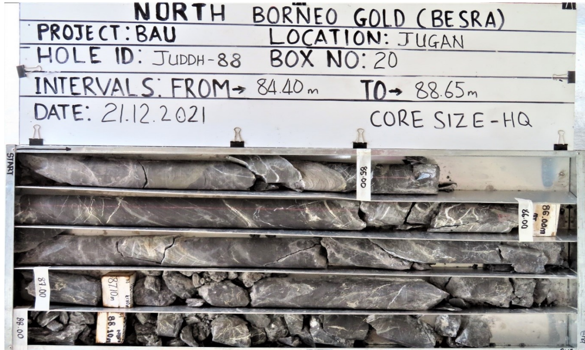
Figure 8: Core recovered from JUDDH-88 for portion of the interval 82m-88m @ 5.98 g/t Au, proximal to the interpreted footwall thrust.
