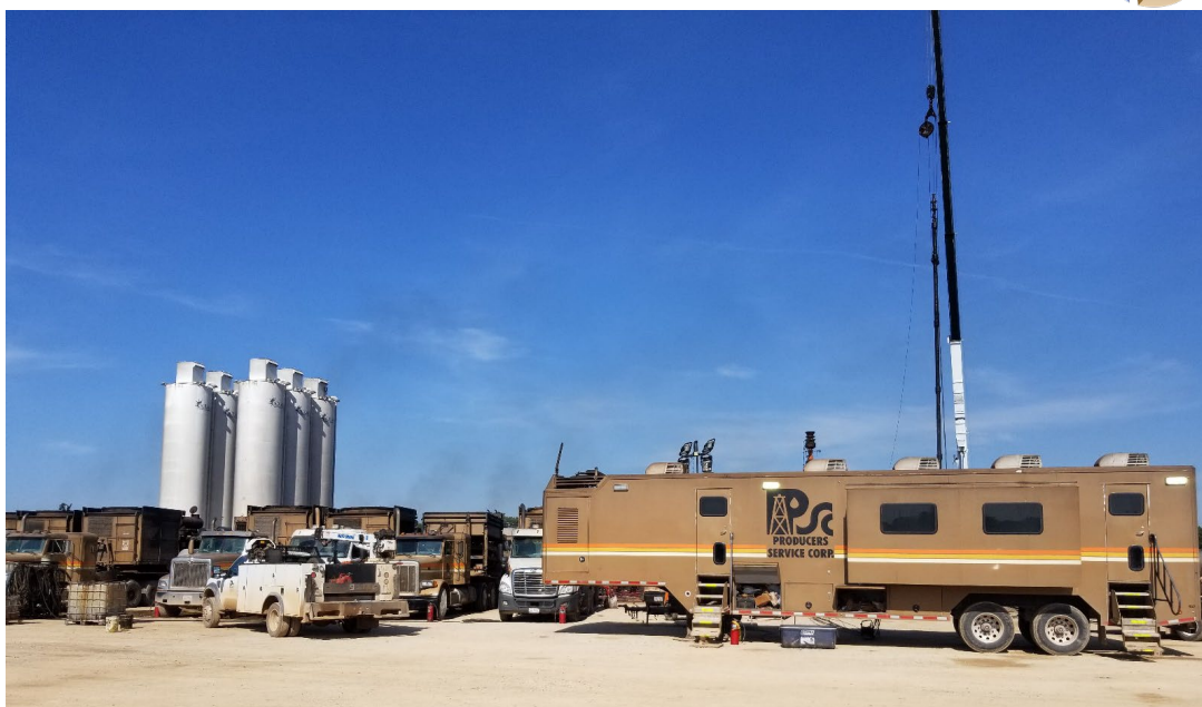
Figure 6. Producers Service Corp. (PSC) conducting multi-stage hydraulic stimulation operations on the Flames Well, Carter County, Oklahoma.
